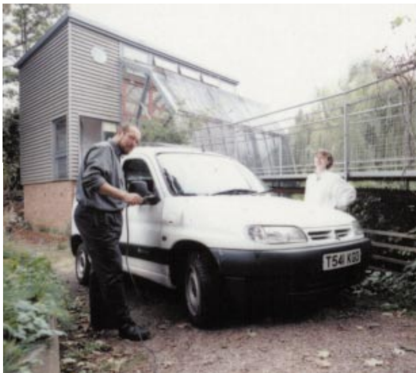
A Citroen Balingo electric van at Hope House, with rear floor pan cut back to fit rear bench-seat, side windows and a sunroof. The cost of the van, enough photovoltaic panels to run it for around 5000 miles/year, and the modifications, are still less than the price of a fossil-fuel-powered people carrier, and the electric vehicle has similar functionality in urban areas
