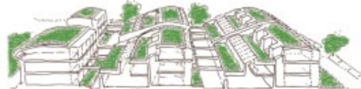
04 – Integrated live/work community: 100 homes and 203 workspaces/ha: With a shared car pool, parking and skygardens placed on workspace roofs enabling the densification of suburbia around public transport nodes without net loss of amenity.
