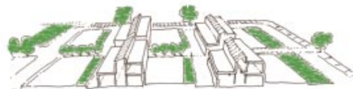
03 – ZEDfactory team propose an additional: 1560m 2 net workspace on the same 0.64 ha plot. Density is 203 workspaces/ha @ 12m 2 /workspace, with car pool shared with housing
